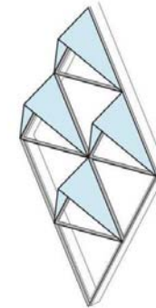
West Façade Shade with no glass
